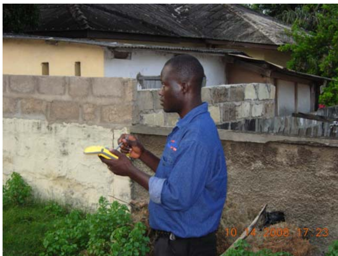
Figure 2: Conducting a property survey using handheld GPS
